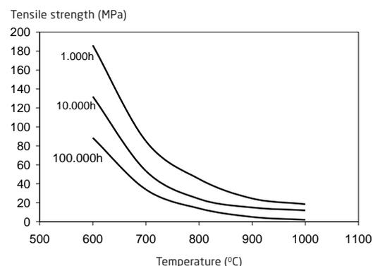
The Figure above shows values of tensile strength in creep deformation test..
